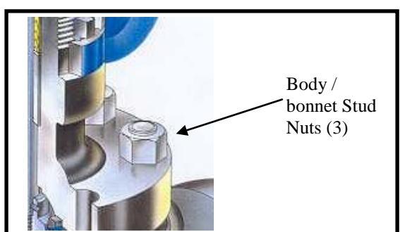
Note: If heat is applied discard studs and nuts after removal.
